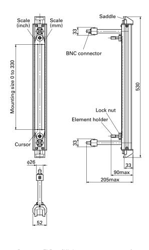
Detector, FLD32 (High-temperature sensor)
