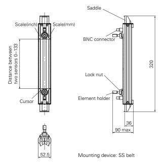
DETECTOR: FLD220 (Small diameter sensor)
